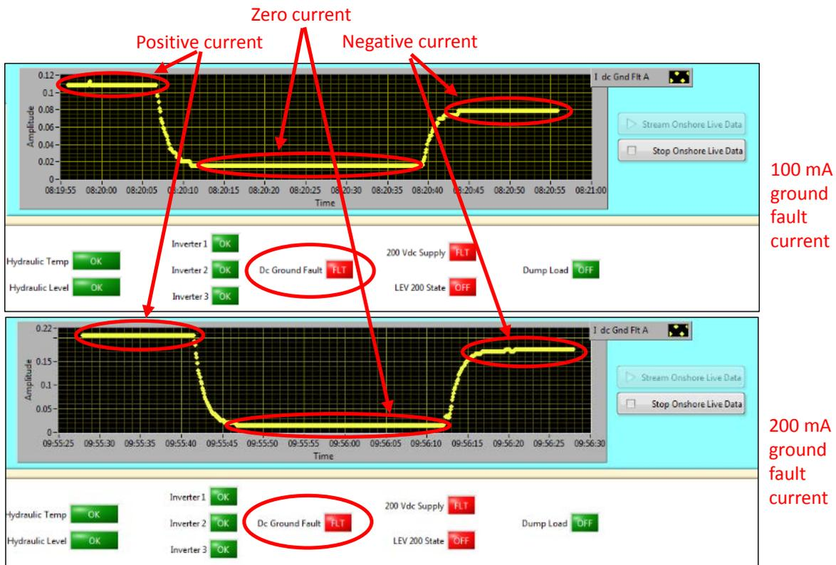
Figure 18 cRIO user interface showing results of 100 mA and 200 mA ground fault tests
