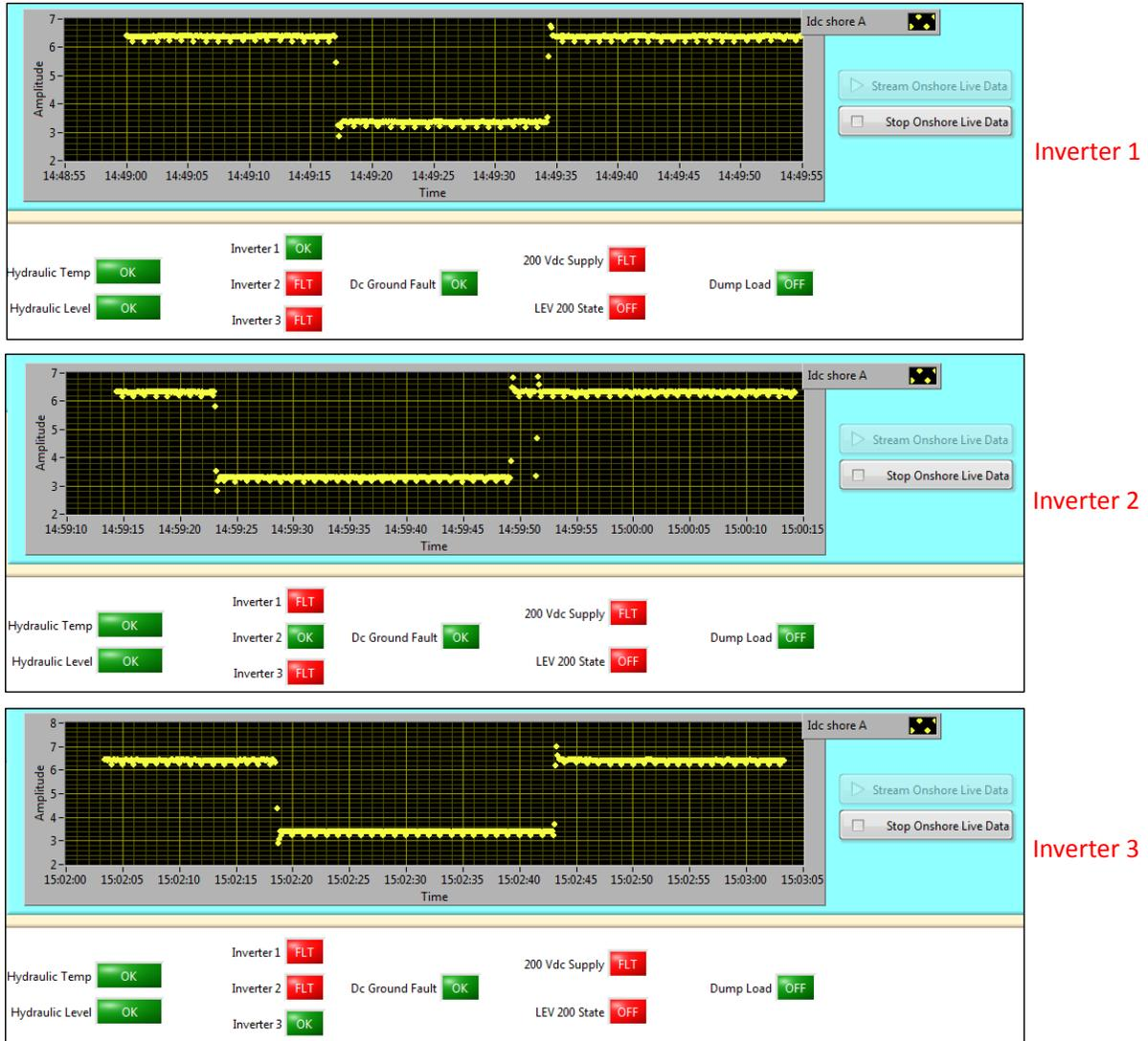
Figure 16 Inverter input currents for individual operation with 3A, 6A, and 3A manual current command
