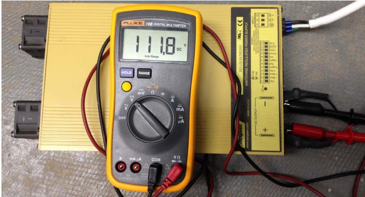
Figure 15 Acopian 0-110 Vdc power supply that was used to provide dc input power to inverters
